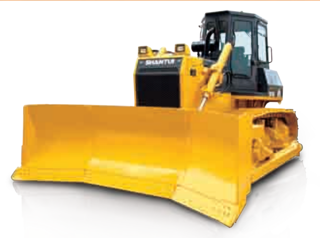
SD16C ▲ Use: Coal Rated Power: 120kW@1850rpm Engine Model: Shangchai SC11CB184G2B1/ Weichai WD10G178E25 Operating Weight: 16.8 Tons
