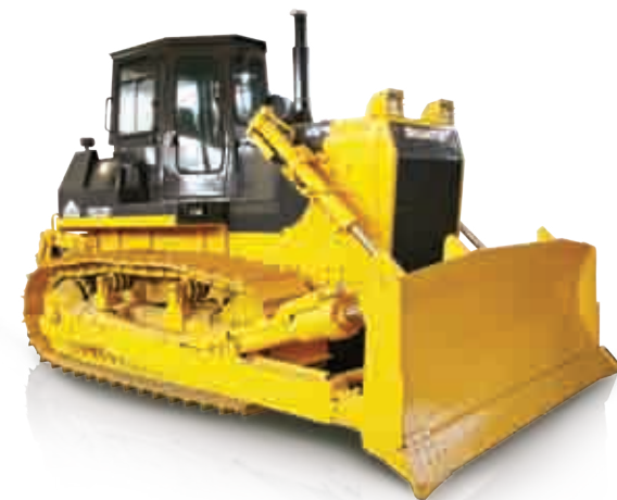
SD22D ▲ Use: Desert Rated Power: 162kW@1800rpm Engine Model: Cummins NT855-C280S10 Operating Weight: 25.8 Tons
