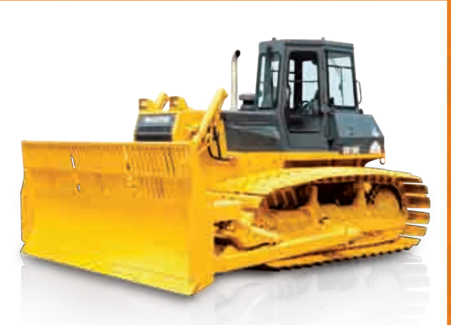
SD16R ▲ Use: Waste Management Rated Power: 120kW@1850rpm Engine Model: Shangchai SC11CB184G2B1/ Weichai WD10G178E25 Operating Weight: 17.7 Tons
