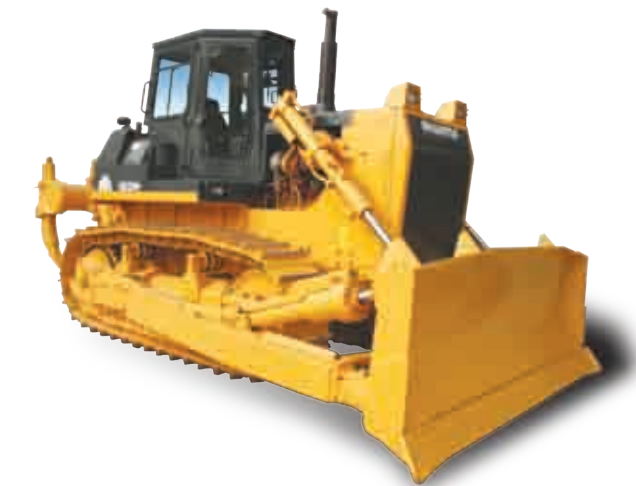
SD22W ▲ Use: Mining Rated Power: 162kW@1800rpm Engine Model: Cummins NT855-C280S10 Operating Weight: 23.44 tons
