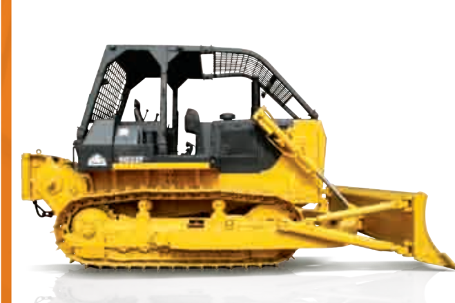
SD22F ▲ Use: Forest Rated Power: 162kW@1800rpm Engine Model: Cummins NT855-C280S10 Operating Weight: 23.4 Tons
