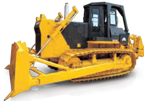
SD32D ▲ Use: Desert Rated Power: 235kW@2000rpm Engine Model: Cummins NTA855-C360S10 Operating Weight: 37.2 Tons
