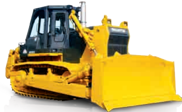
SD32W ▲ Use: Mining Rated Power: 235kW@2000rpm Engine Model: Cummins NTA855-C360S10 Operating Weight: 38 Tons
